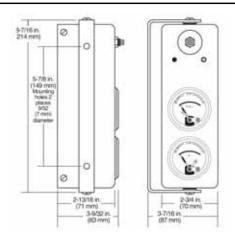
It is the ability of this panel to mount in many different positions (Swichgage instruments can be rotated, the panel tilted) that allows for instrument visibility without a difficult installation or interference with other engine equipment.
